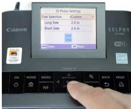
5. The printer defaults to the Custom 2.0 x 2.0 inch print size. Press the OK button to confirm size.
