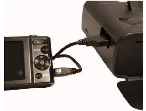
3. Use the USB cable to connect the camera's small USB port to the USB port of the side of the printer.
