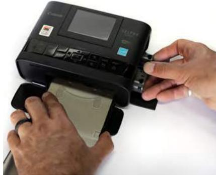
2. Ensure paper is in paper tray and an ink ribbon cartridge is in the printer.
