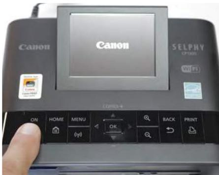
4. If not already powered on, turn printer on by pressing the ON button until you see the Canon logo on the LCD screen.
